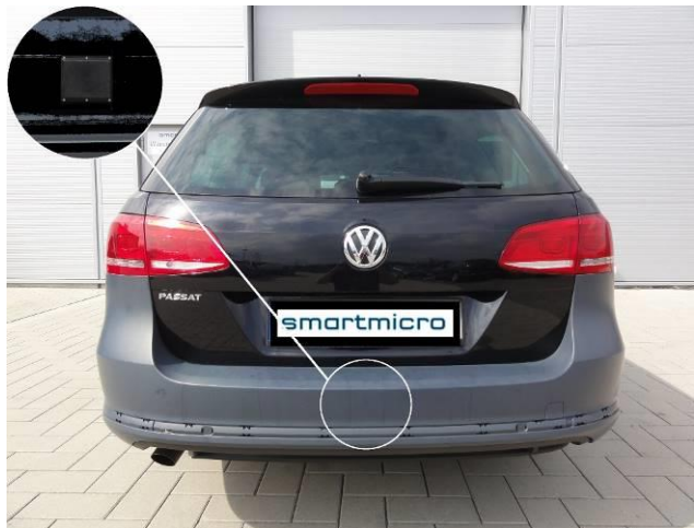
Sensor mounted behind the bumper
